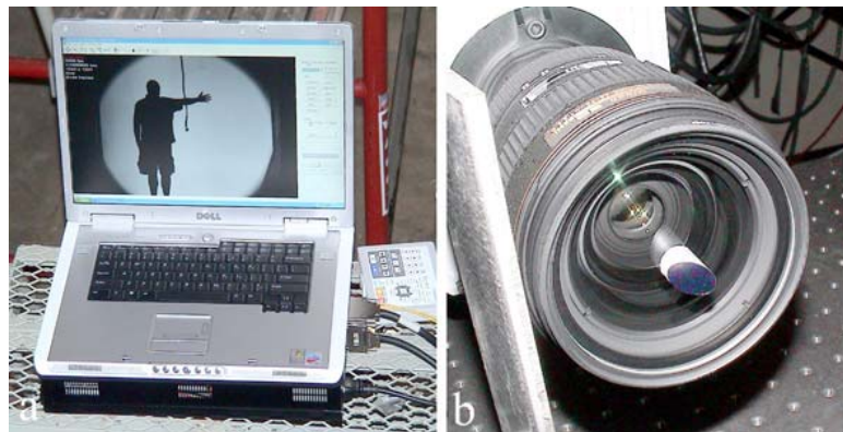
Figure 3. a) Real-time shadowgram image on laptop computer controlling the APX-RS digital video camera. b) APX camera and zoom lens with clear filter and rod mirror installed.
