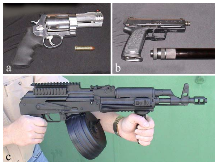
Figure 7. Three of the firearms tested here: a) Smith & Wesson .500 Magnum revolver, b) Heckler & Koch USP Tactical pistol, .45ACP, firing American Eagle ammunition, shown with B&T ImpulsII-A suppressor, c) AK-47 submachine gun with 30 cm barrel, firing 7.62x39 ammunition.
