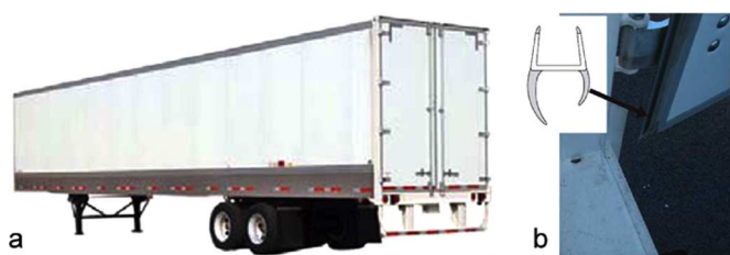
Fig. 3. (a) A 16.15 m (53 foot) truck-trailer with a van-body style and swinging doors. (b) The swinging doors have seals on all four sides with the seal geometry shown in the inset. When closed, the seal compresses and a central air passage is created around the perimeter of the door.
