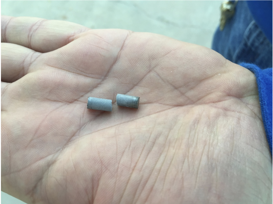
Figure 4.11: Al/I 2 O 5 thermite pellet after test, found mostly intact
