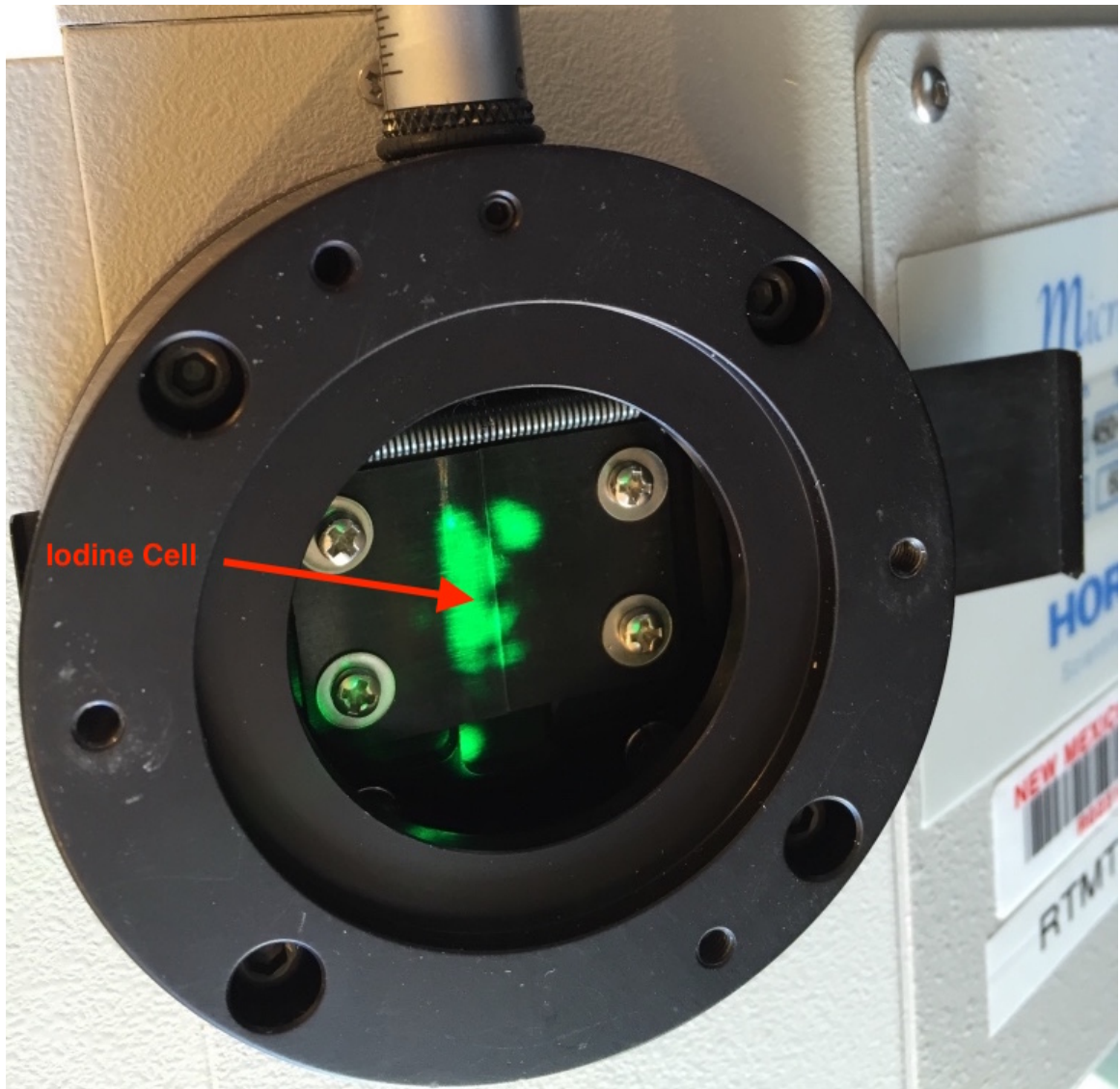
Figure 3.10: Light incident on spectrometer entrance slit. The circular shadow in the center is the iodine cell.
