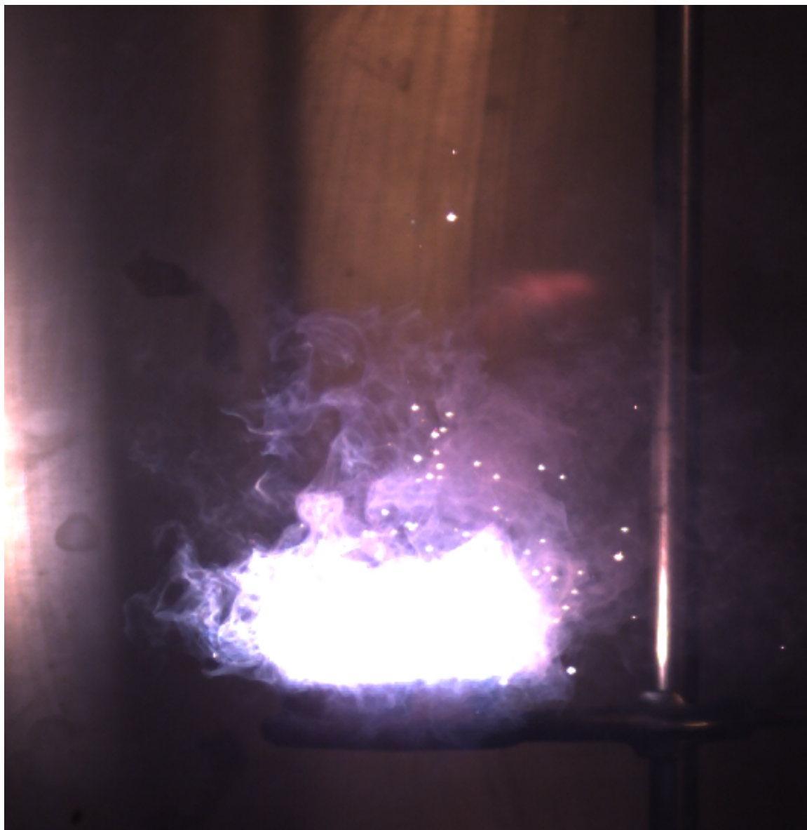
Figure 2.8: Initial test of 2.5 grams Al/I 2 O 5 thermite
