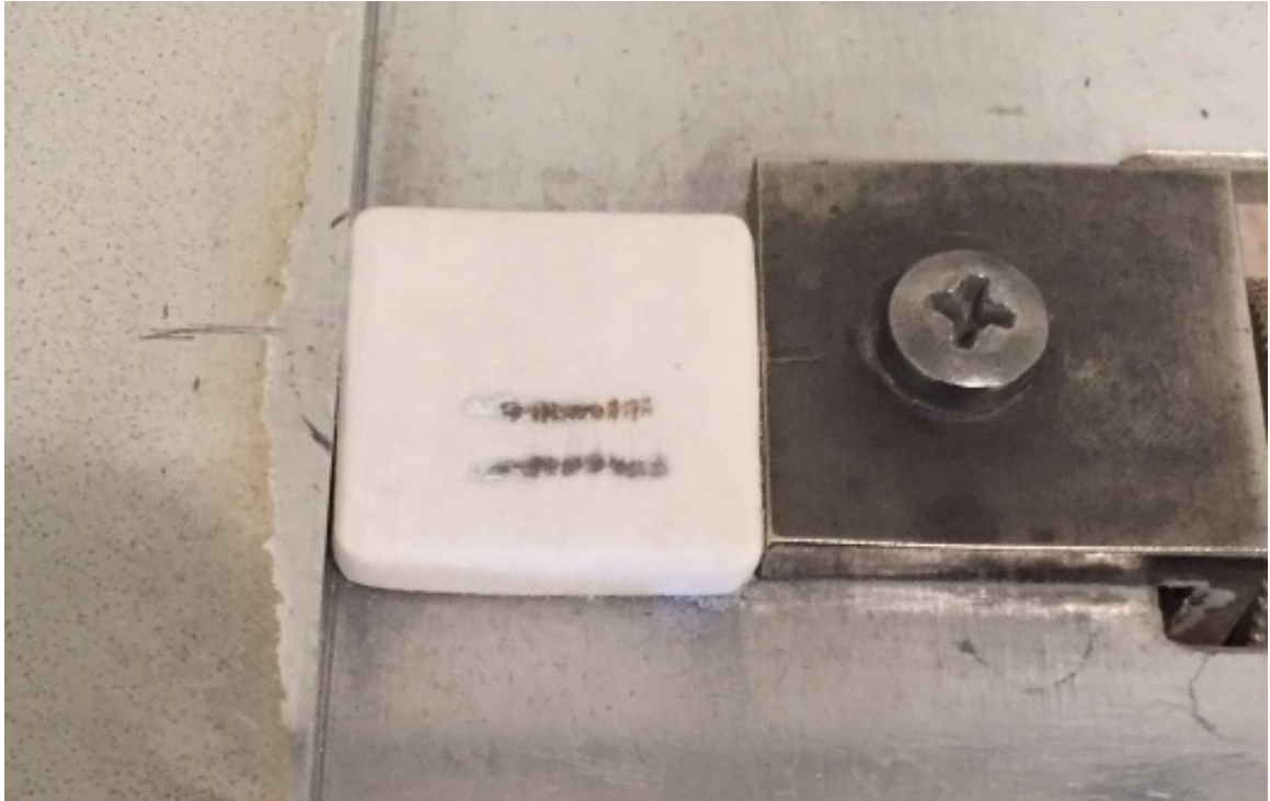
Figure 2.2: BAM Friction Sensitivity Apparatus setup and indication of a go vs. a no-go (determined by the purple remnants on the plate on the top test)
