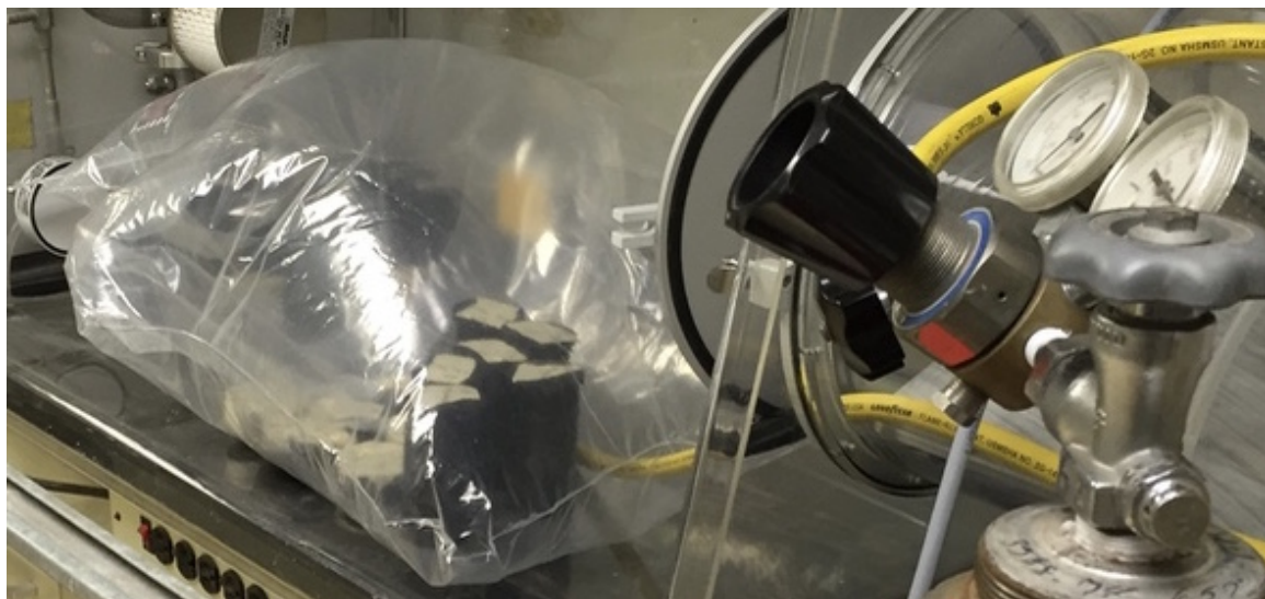
Figure 2.9: Storage of Al/ I_2O_5 thermite under nitrogen for aging study
