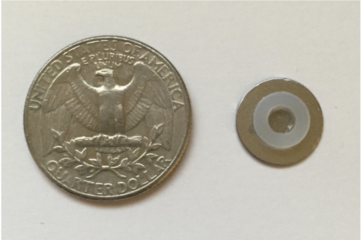
Figure 2.4: Static-Spark Sensitivity test cup - The explosive being tested is placed in the inside of the plastic washer, with enough material to fill the entire cylindrical volume
