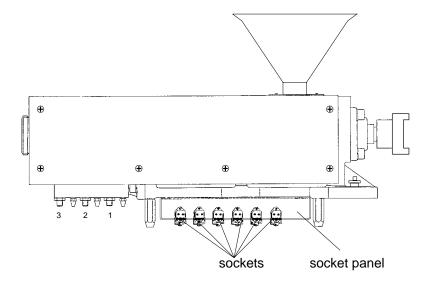
A socket panel on the right side of the extruder is provided for connecting a die with several heating connections.
