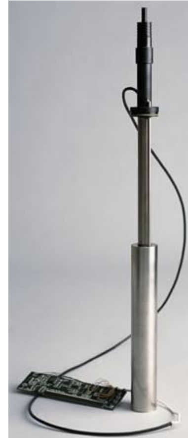
4mL minicalorimeter attached to its computer interface
