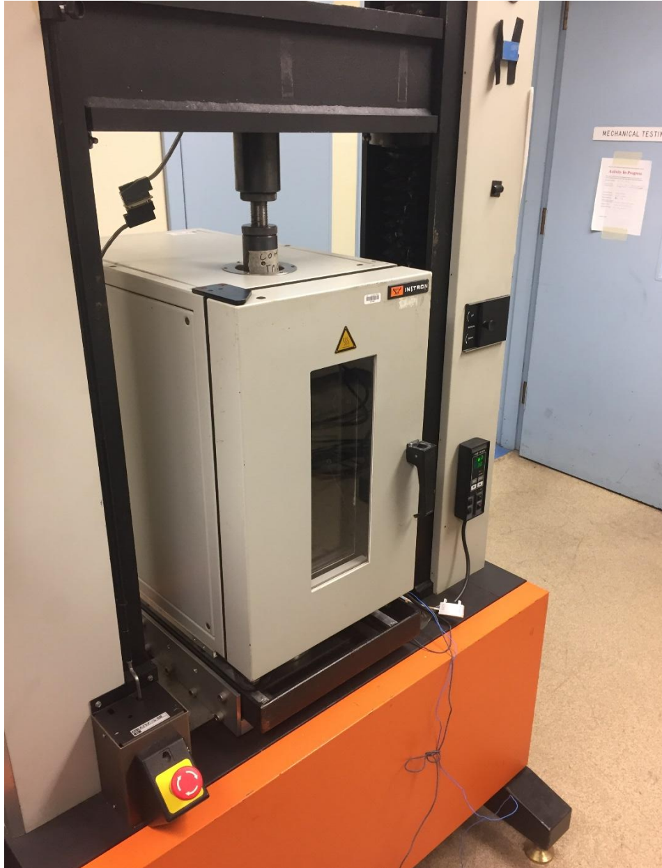
Emergency off button and circuit breaking pins
