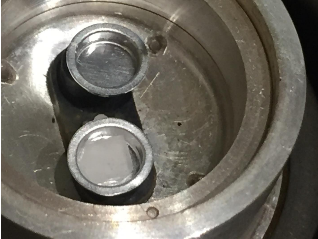
Figure 10. DSC sample chamber with sample pan and reference pan.
