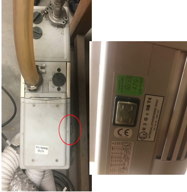
Pump switch on side of pressure chamber
