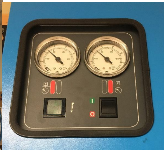
Figure 4: The Hankison’s power switch and air pressure gauges.
